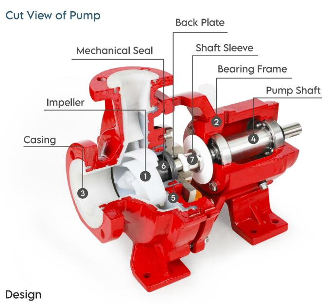
Single stage, plastic lined, frame mounted chemical process pump of heavy duty design. Flanges with holes drilled to ANSI B16.5 CI.150.
